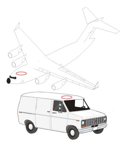
This illustration provides examples of where the antenna may be located on an aircraft or vehicle (not to scale).
