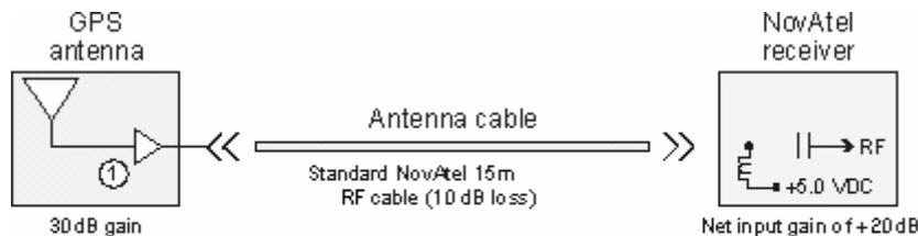
① The antenna LNA is powered by +5.0 VDC from the receiver via the antenna cable center conductor.
