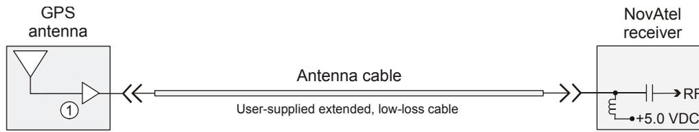
① The antenna LNA is powered by +5.0 VDC from the receiver via the antenna cable center conductor.
